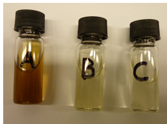
Fig. 3. TMP-trioleate sample product obtained using (A) silica-sulphuric acid, (B) Amberlyst 15, and (C) Novozym®435. The Gardner index for the samples was 5, 3–2 and 2, respectively.
